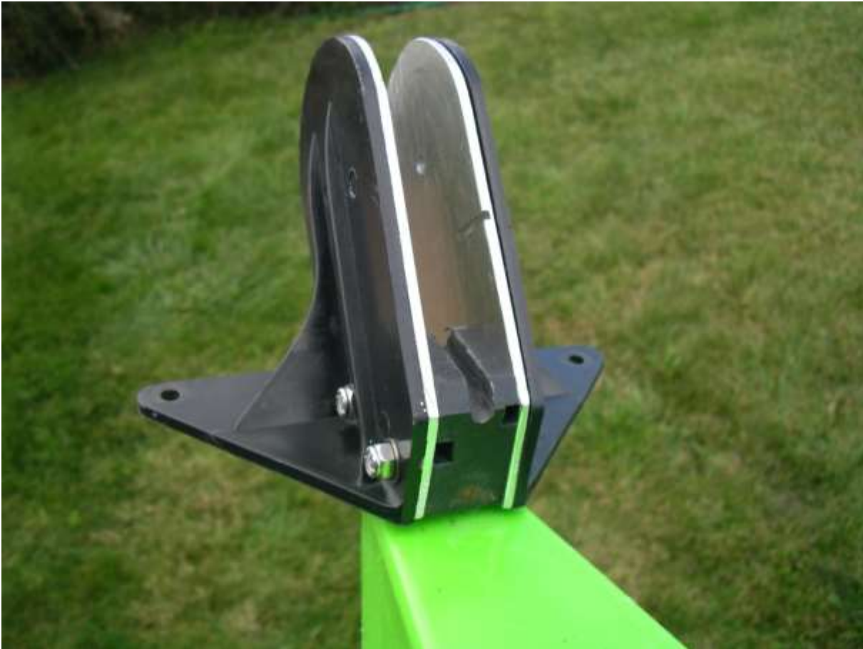
Stopped the plastic cheeks twisting.
