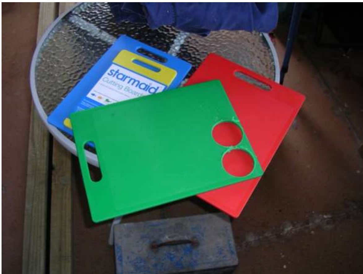
Cut new spacers with a hole saw.
